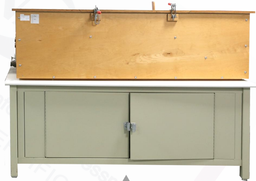
UL Smoke Chamber
